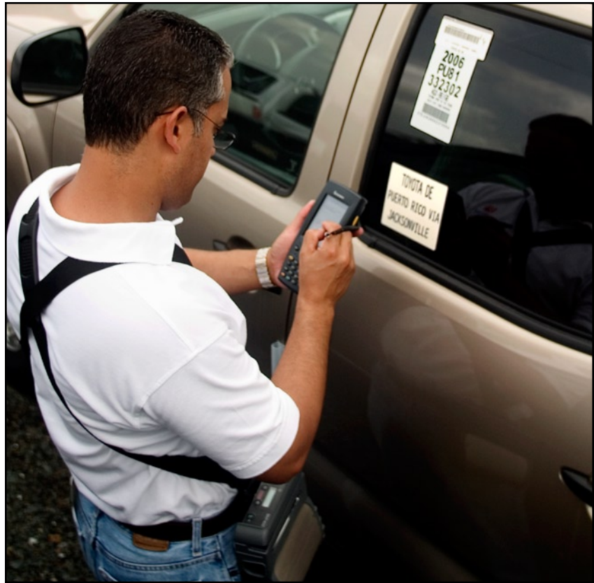
Labels produced on the MtP400LP printers are affixed to the outside of vehicles and must remain readable up to 10 months despite exposure to sun and rain.
